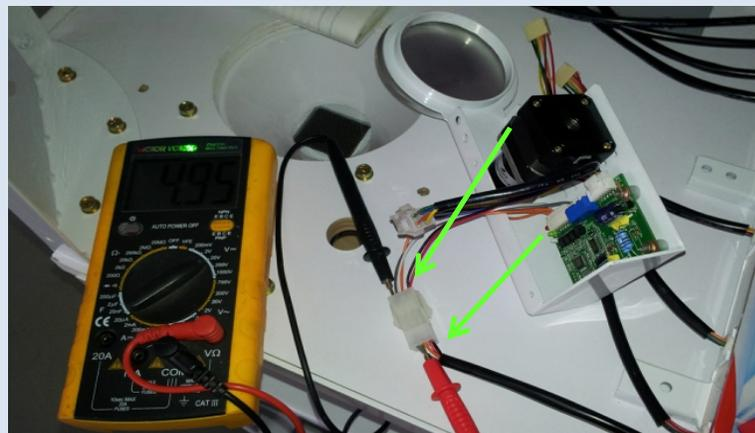
**Step #8 Replace the Motor driver board.**
